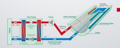
Centerpiece is the heat exchanger in variable shape, designed for maximum heat transfer performance. All components to be installed in the sewer are made of stainless steel and are protected against the detrimental fouling effects by a patented method.
