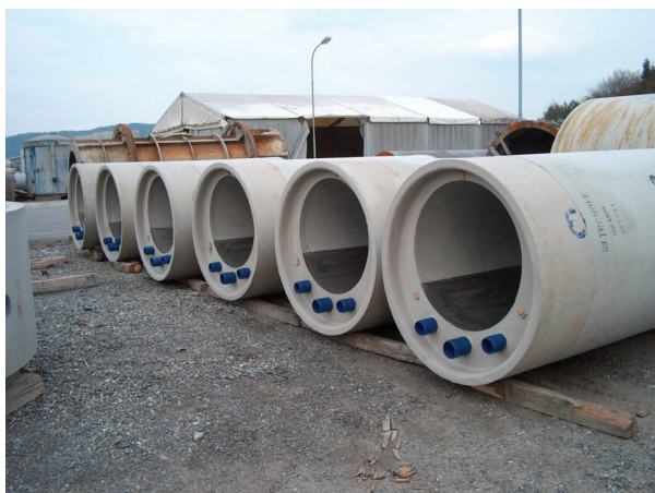
Heat exchangers are integrated into sewer pipes in order to extract heat from wastewater
